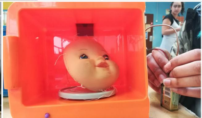
When you switch on this project, the baby face starts to turn, there is light in its eyes and some gloomy music can be heard. This project re-used motors, LED, speakers, resistors, and switches.
