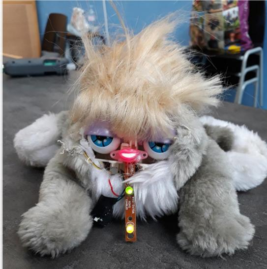
When switched on, the eyes start to move and lights blink. This project re-uses motors, LEDs, switches and resistors.
