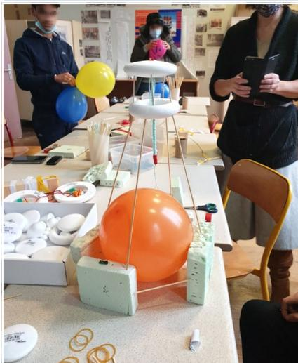
Toothpicks are taped on the balloons and attached to the string. The balloons are attached to something heavy or the table so that they do not move. When the string is pulled away, the toothpicks move and pop the two balloons simultaneously.
